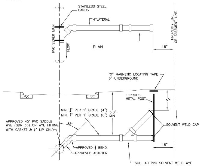
NOTE: ANY LATERAL OVER 10.0 FT. IN DEPTH WILL BE RESTRAINED JOINT DIP 4" AND 6" LATERALS
