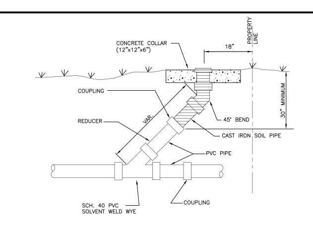
NO HUB STAINLESS STEEL BANDS REQUIRED BY DURHAM COUNTY 3 \$\frac{1}{4}\text{"} X PIPE DIAMETER OR GREATER PER PIPE SIZES
