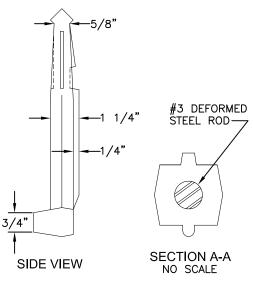
DIMENSIONS OF STEPS MAY VARY DEPENDING ON MANHOLE WALL THICKNESS AND TYPE OF CONSTRUCTION.
